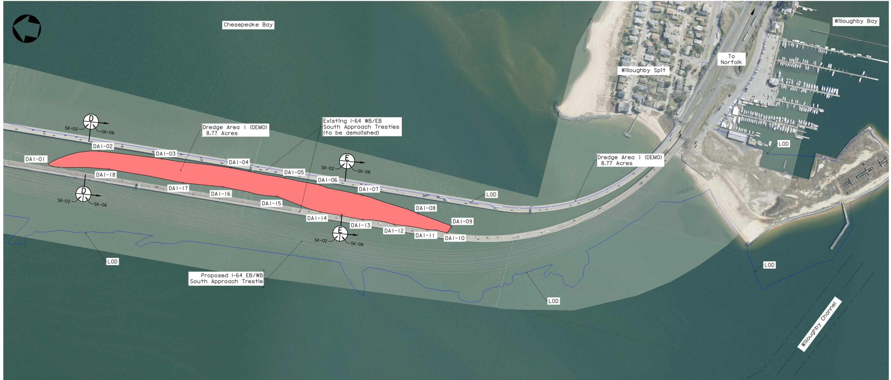
SOUTH TRESTLE DREDGE PLAN - DEMOLITION AREA Scale: 1" = 400'
