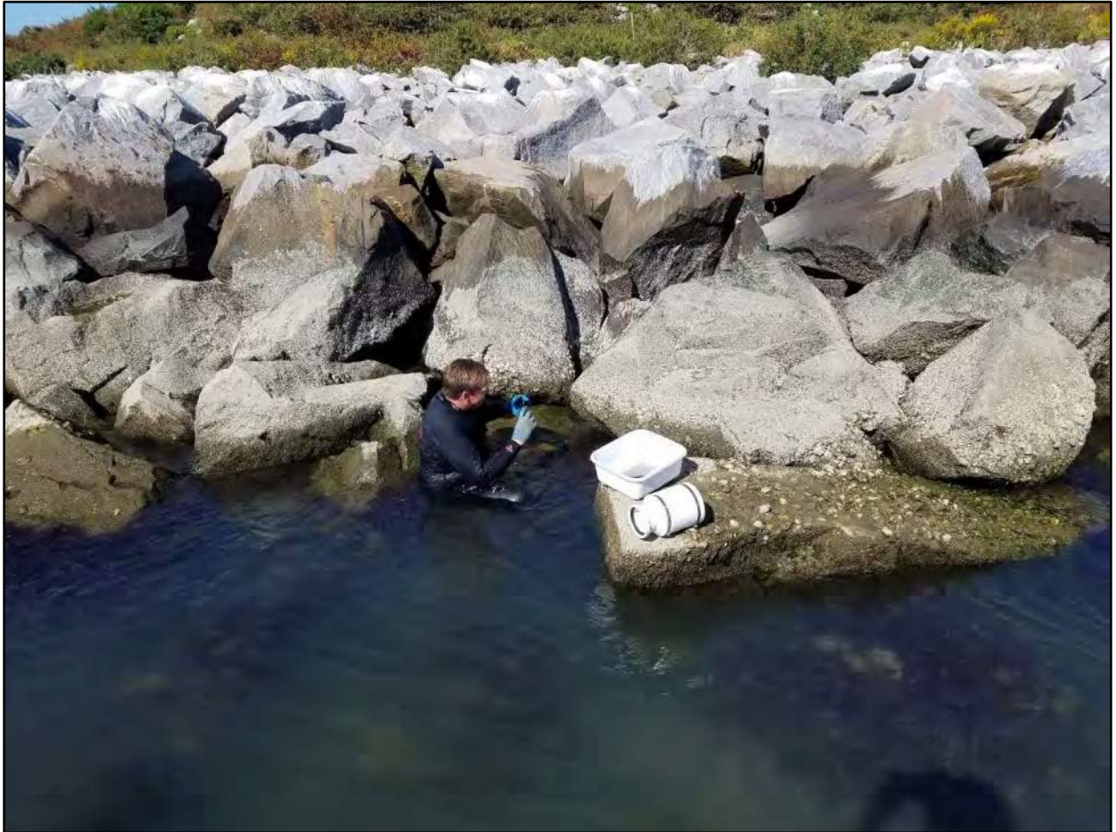
Figure E-2. Diver taking photographs of an intertidal site prior to sampling. The piece of PVC in this image was used to mark the sample areas to be scraped
