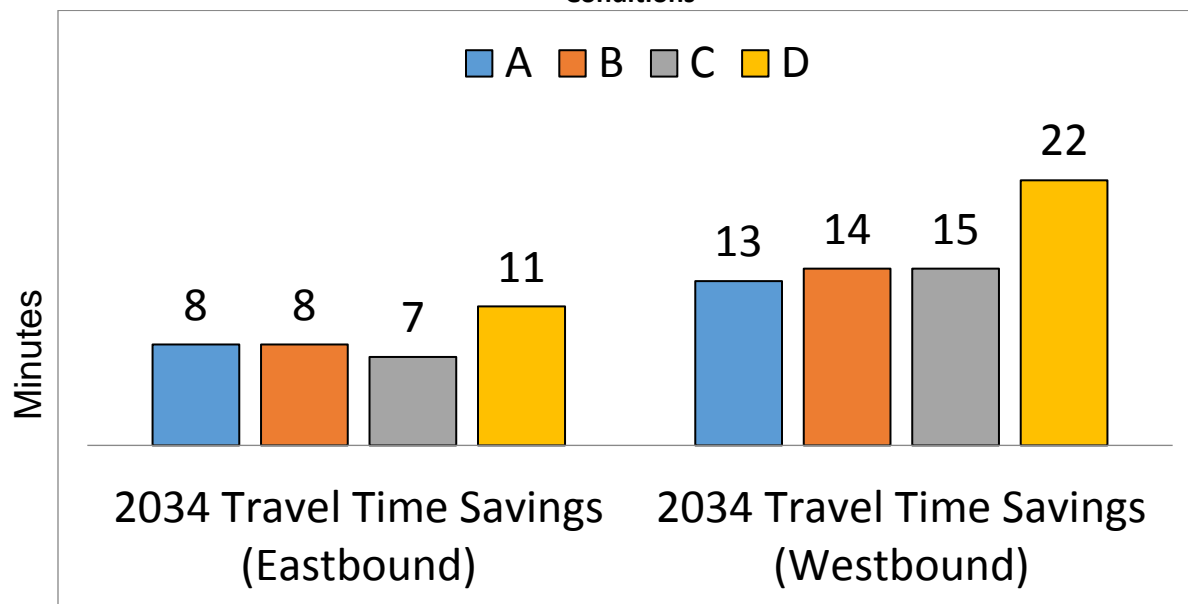
Figure 2-22: 2034 PM Peak Hour Travel Time Savings along I-64 HRBT Compared to No-Build Conditions
